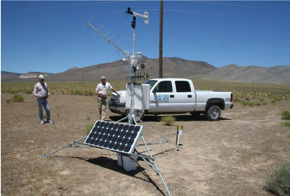
Figure 3. The Smoky Site CA meteorological station was installed to measure precipitation, wind, and other climate parameters. A radio communication system is used to exchange information with the flume datalogger and the Geostationary Operational Environmental Satellite (GOES) communication system allows regular data transmission to the Western Regional Climate Center (WRCC) in Reno.
