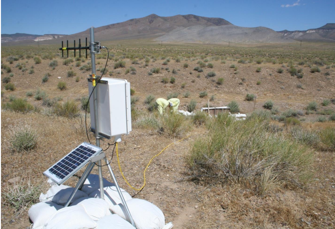
Figure 5. Runoff conditions in the flume are detected by the pressure transducer and transmitted to the datalogger (inside the white enclosure) via the yellow cable, recorded in the datalogger, and relayed by radio (black antenna) to the meteorological station. (Since this photo was taken, the pressure transducer cable was placed in a conduit to protect it from damage by animals.)
