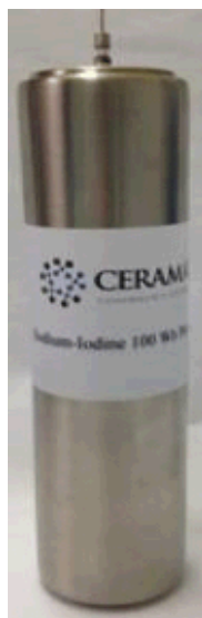
100 Wh, Na-battery prototype
