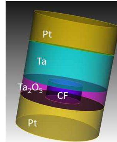
*Memristors switch between low and high resistance states*
