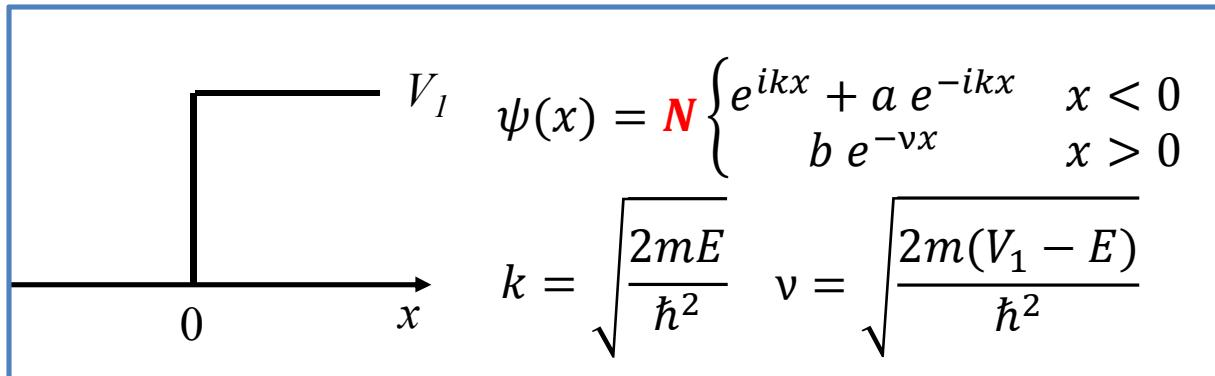
Consider  $0 < E < V_1$  and  $x > 0$  (relevant for b-to-t tunneling)
