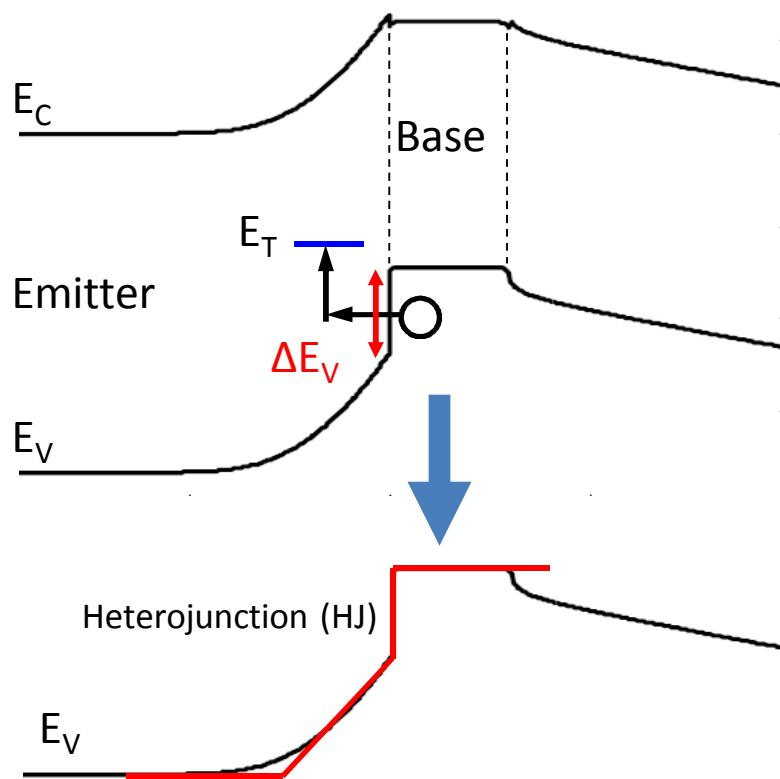
DOS at the trap location is **greatly enhanced** [5] due to the **band offset**  $\Delta E_V$ , leading to much **higher hole-to-trap tunneling**.
