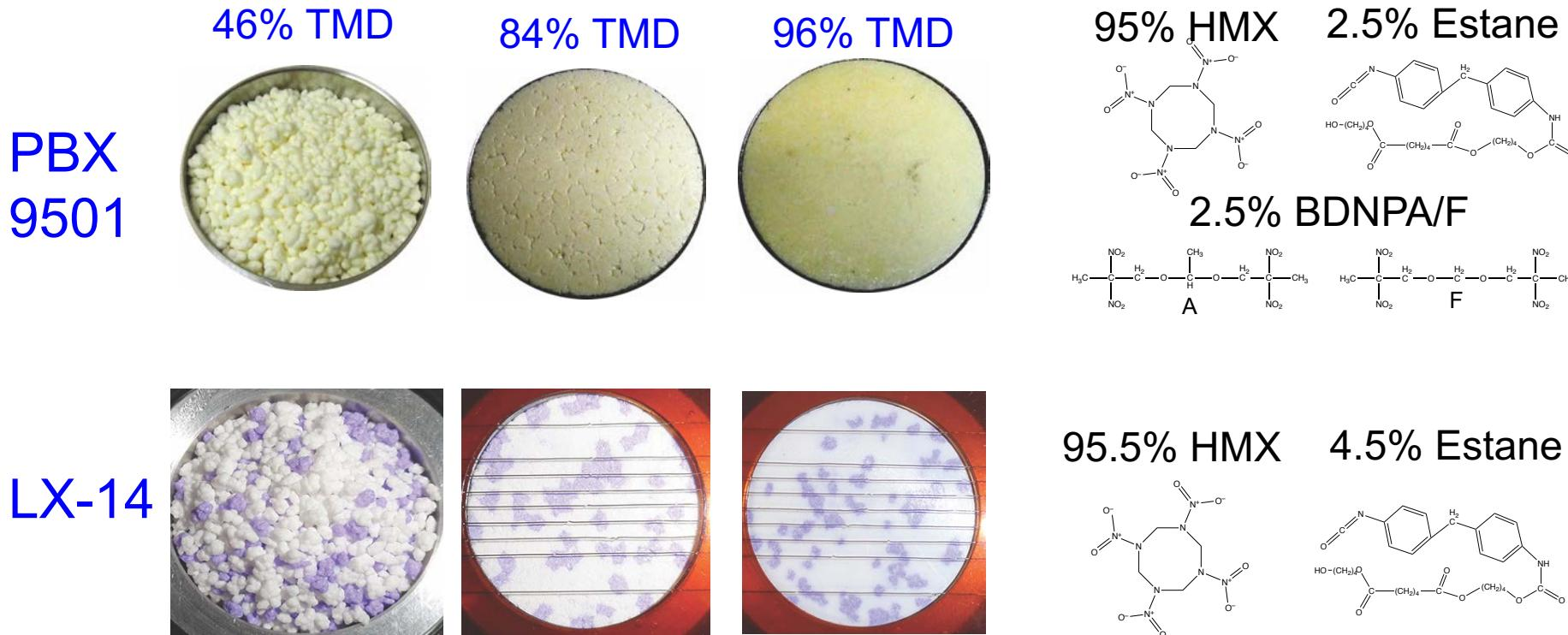
*These explosives have nominally the same detonation performance and give the same flame temperatures. However, the LX-14 reacts sooner in cookoff tests and is more violent in blunt impact tests.*
