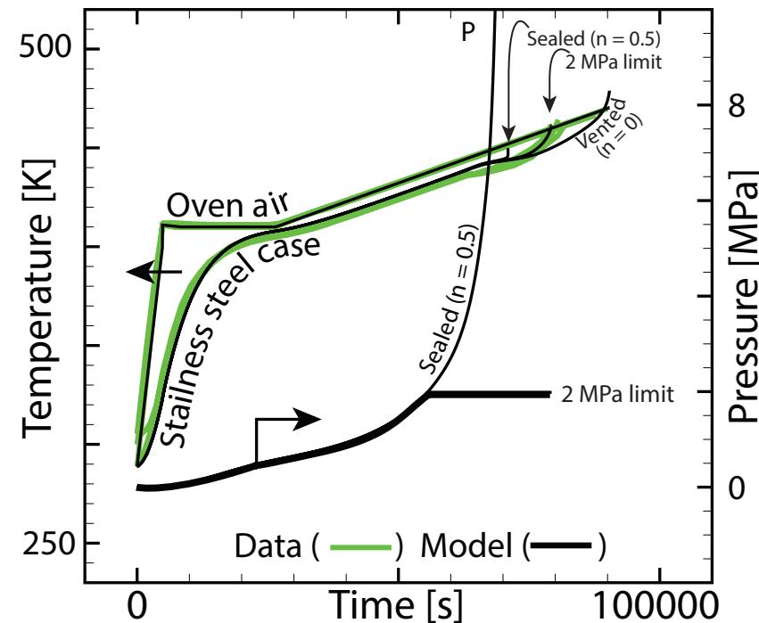
Vented model ( $n=0$ ) and sealed model ( $n=0.5$ ) bound data. Setting working pressure of confinement to 2 MPa matches data.
