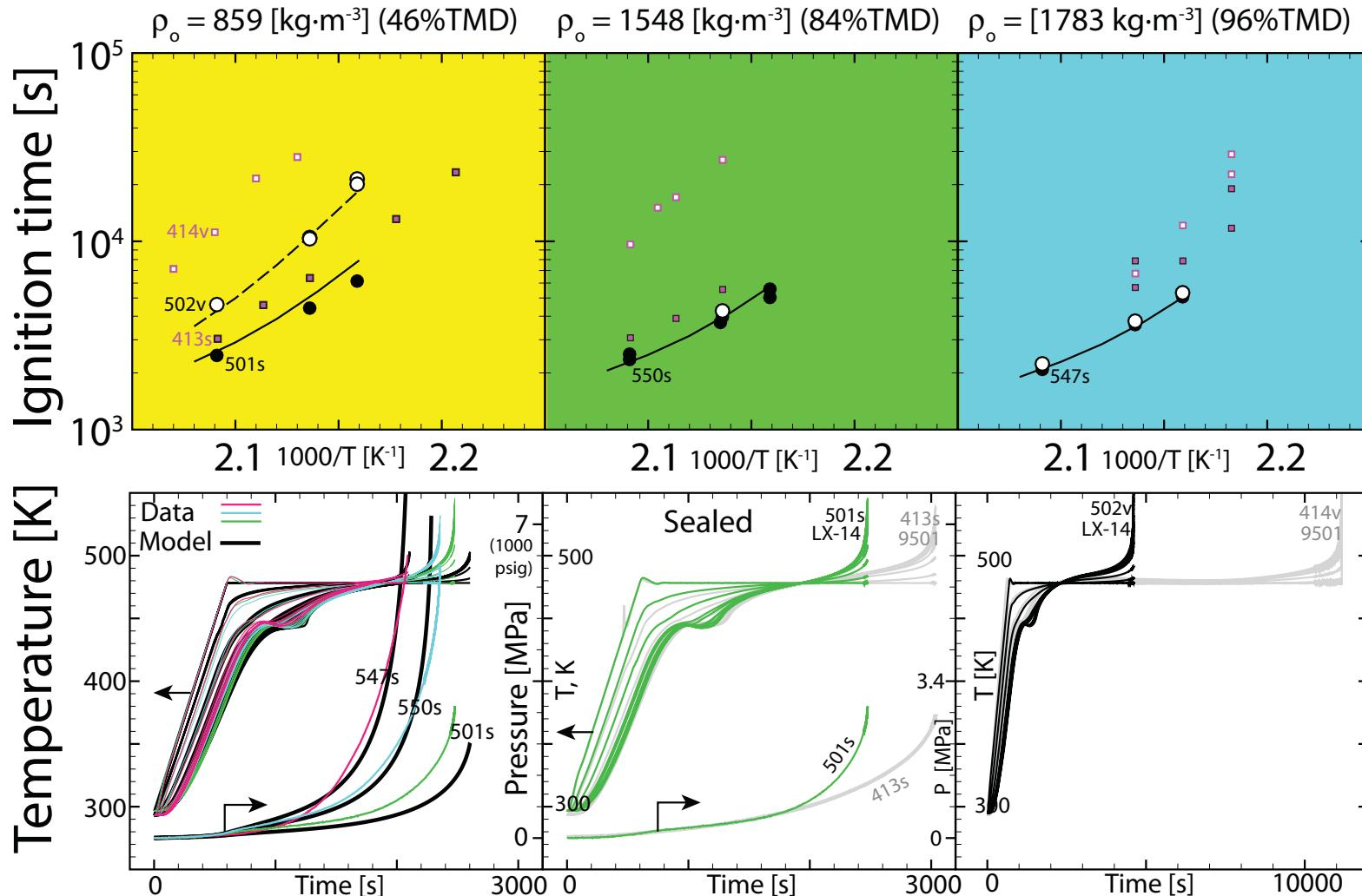
*Model matches ignition time, internal temperatures, and pressure. The effect of venting on LX-14 is significantly less than with PBX 9501.*
