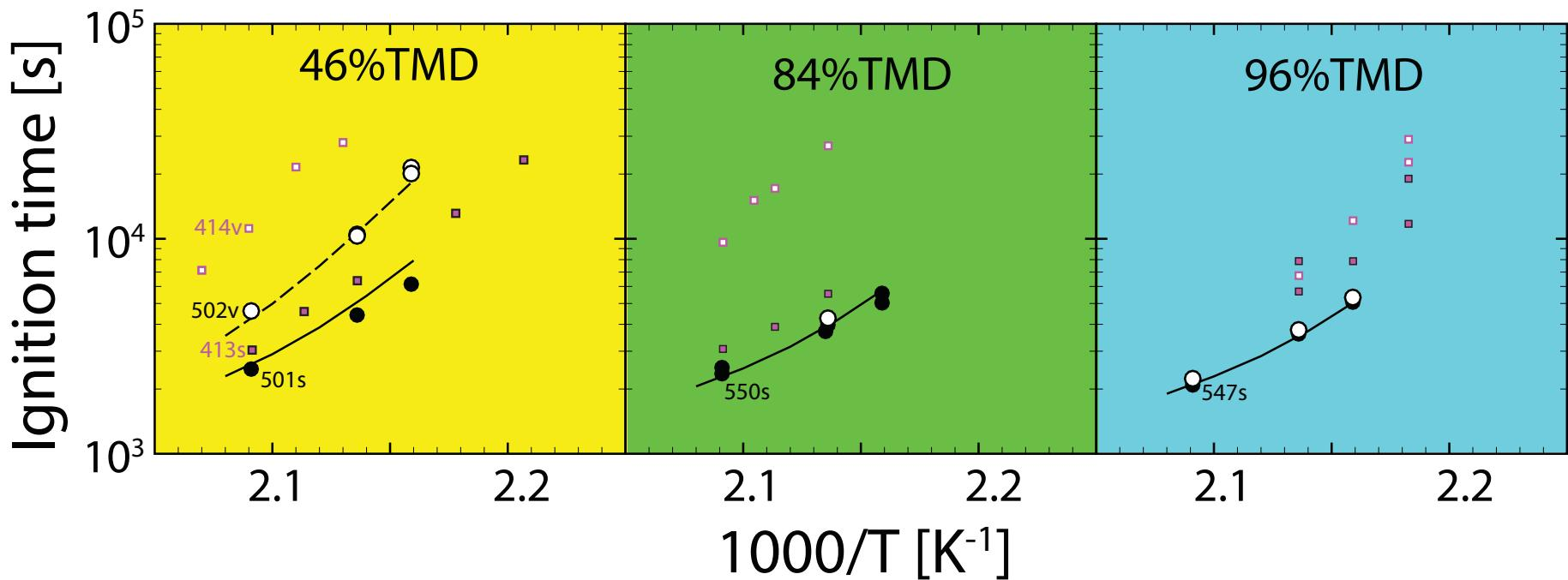
*PBX 9501 ignition delay due to venting is significantly greater than for LX-14. Venting does not affect LX-14 for densities greater than 84% TMD (1.5 g/cc).*
