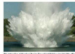
This detonation at Aberdeen Proving Ground last October simulated the effects of a nuclear blast in a ship's hull.
