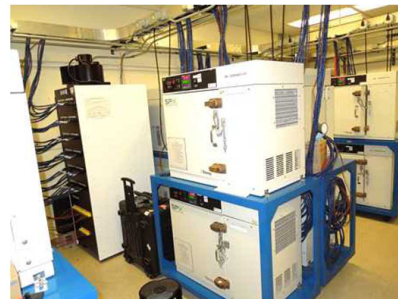
Battery aging facility; ~400 channels dedicated to lifetime monitoring of batteries under environmental conditioning
