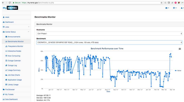
Figure 4. NERSC Benchmarks Monitor dashboard showing performance of a benchmark on the CSCRATCH file system. Occurrence of performance degradation is clearly seen.
