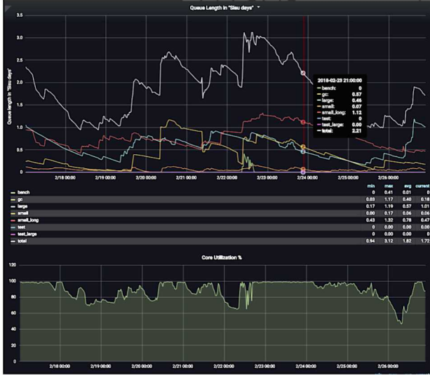
Figure 13. CSC Sisu job queue length development over 7 days. Occurrence of high priority jobs (yellow queue) and their effects on the throughput of other queues can be seen.
