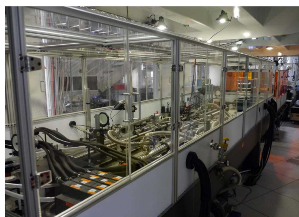
Pulsed laser used for hCMOS x-ray characterization studies
