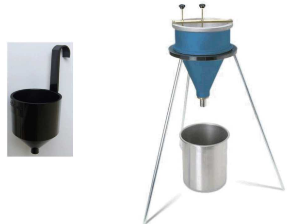
Ford cup (ASTM D-1200) and flow cone (ASTM C-939) testing apparatus:
