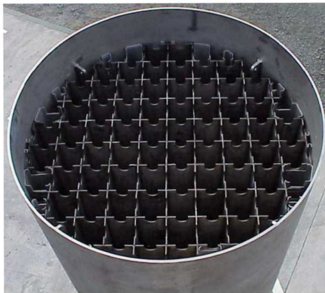
Top view of MPC-68 shell and basket (Greene et al. 2013).
