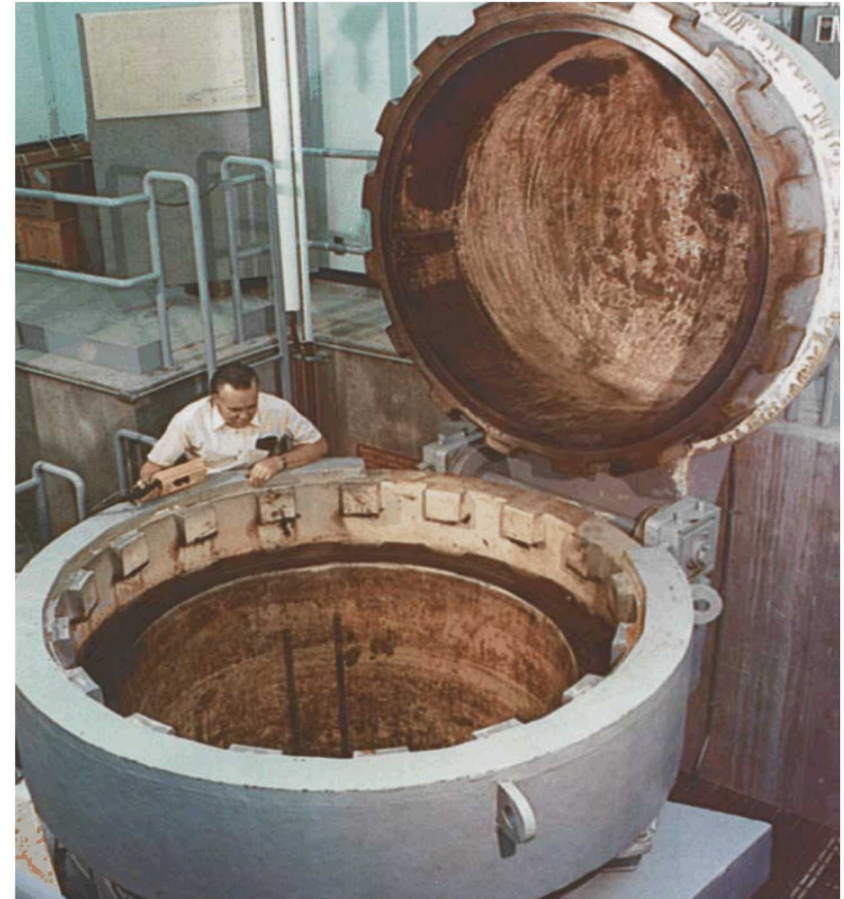
Hydrostatic testing vessel, AECL/Whiteshell
