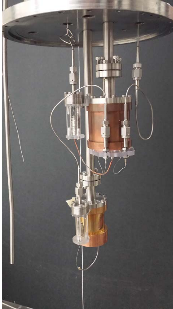
Figure 5. Photo of the cold stage of the helium-three refrigerator. The upper reservoir is the continuous-flow 1 K pot, with a capillary to the left bringing liquid in from the outer bath. The second capillary supplies the returning helium-three gas, to be condensed and delivered to the helium-three pot at the bottom. Both pots are pumped through the stainless-steel tubes to which they are attached.
