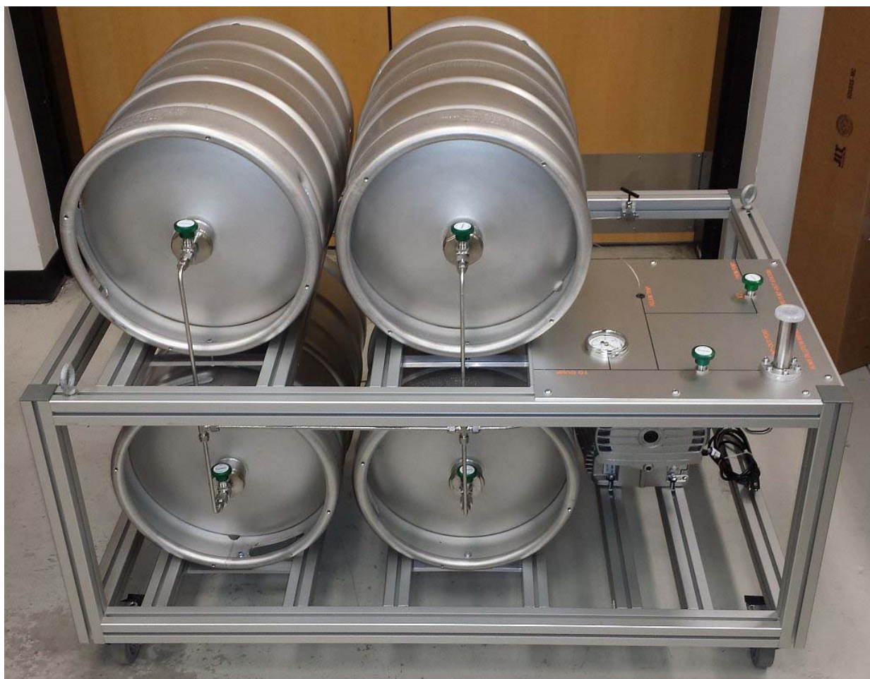
Figure 4. Photo of the ADMX mixture pump out station. The sealed pump may be seen under the panel on the right. There are four storage tanks and manual valves to configure the pumping system.
