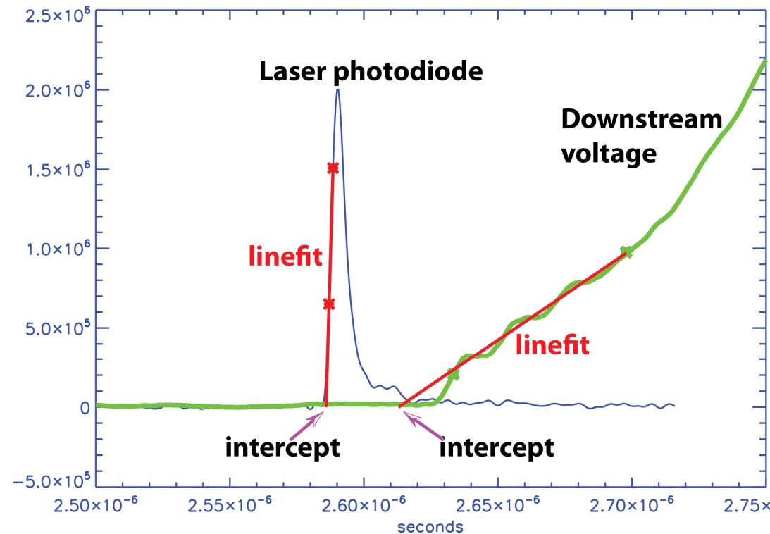
Laser triggered gas switch run time calculation
