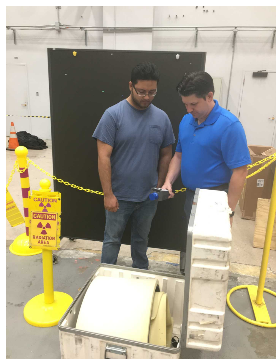
TRB interns use a handheld radiation detector to scan for the presence of radioactive isotopes.
