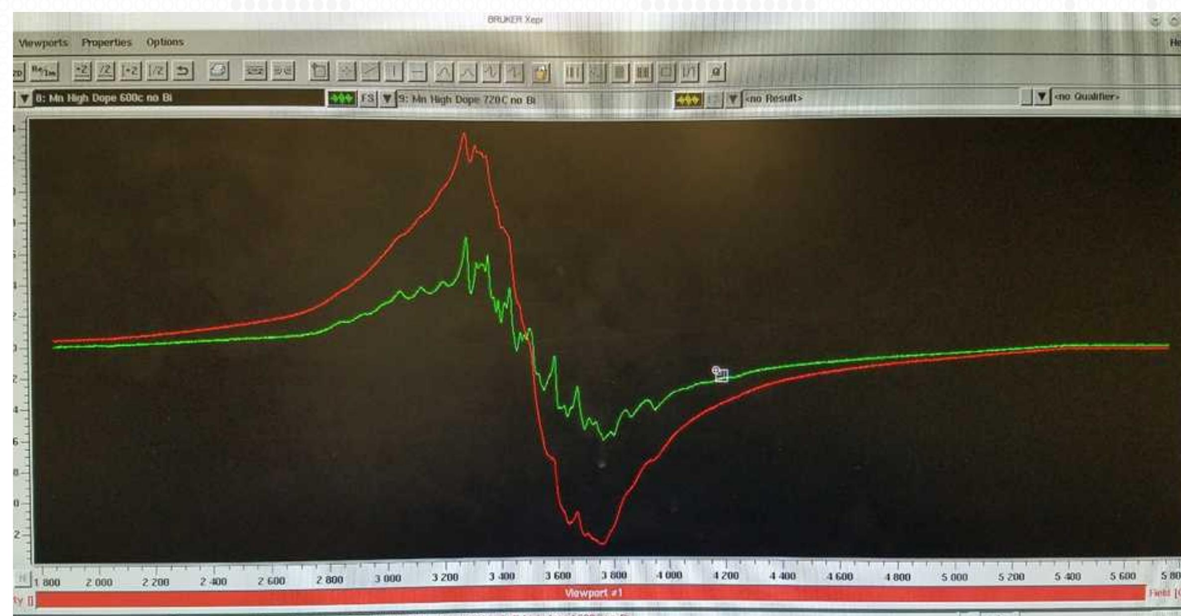
Example shows raw data of two different powders calcined differently with high amounts of Mn: green corresponds to  $Mn^{2+}$ , red is unknown. The fact that both patterns are different tells us that Mn is behaving differently during calcinations
