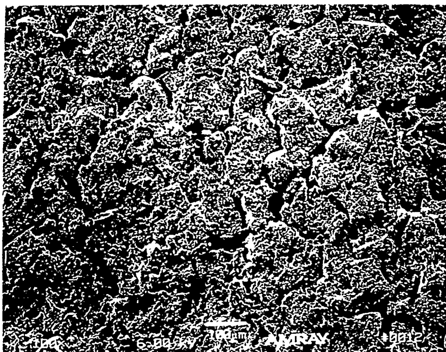
Figure 4. SEM Microstructure of As-Formed Surface of Composition 1-300 @ 100X Magnification
