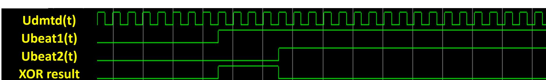
In the figure above, the XOR result is '1' for 4 clock periods of  $u_{dmtd}(t)$ , each of which lasts 50.394 ns (based on 20 MHz input signals). We refer to this XOR result as 'count'.
