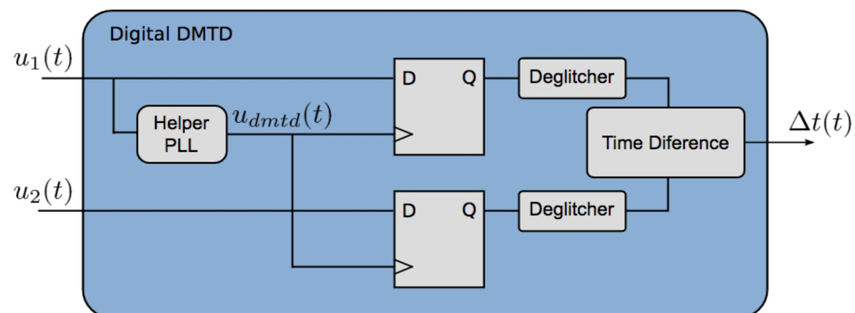
The design consists of two input digital clock signals— $u_1(t)$  and  $u_2(t)$ —both of which have a frequency of  $v_n$  and a relative phase difference of  $\Delta t$ . The Helper PLL is set by the user at a specific frequency to produce the  $u_{dmtd}(t)$  clock signal. To specify  $v_{dmtd}$  use the following formula:
