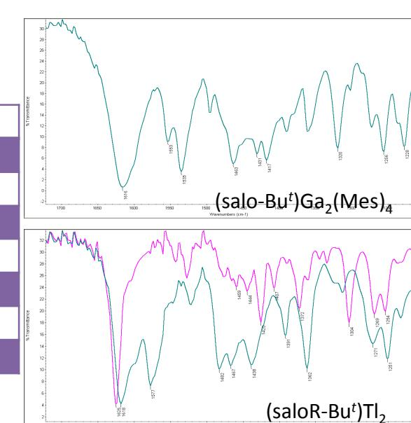
Analysis of metal-salens and salen ligands using Raman and IR spectroscopy show that it is possible to distinguish the ligand to the metal complexes by the carbon to nitrogen stretch in the molecule. In addition to this, there is a varying shift between metal complexes with the same ligand but different metal and also between same metal and different ligand. This gives allows us to pinpoint which metal complex is present in a sample by two simple spectroscopy methods.
