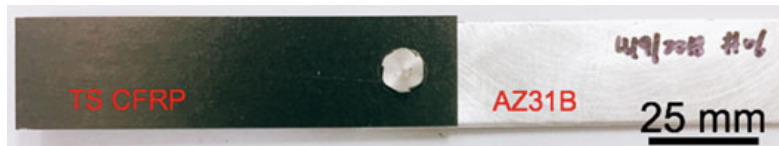
Fig. 4 Example of thermoset CFRP joined to AZ31B by friction self-piercing riveting
