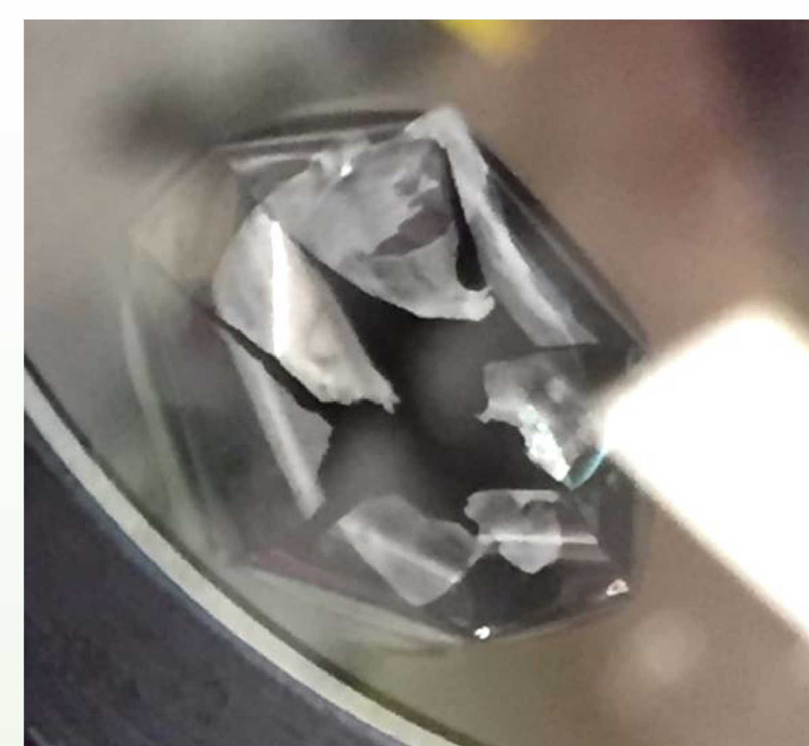
Damage on a 2-μm thick polyimide pellicle. The foil ruptures along the star-shaped focal pattern.
