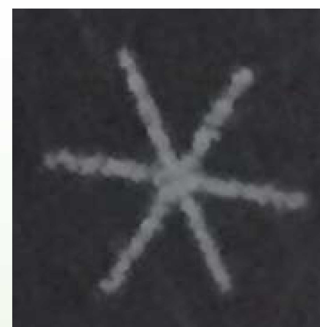
Burn pattern on anodized aluminum. 2 shots on target.
