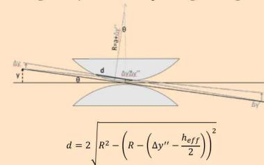
To translate to the object place we scale to  $\Delta y' = (M+1) \Delta y'' / M$ . From the calculated path lengths and the known mean free path,  $\lambda$ , the expected transmission of the slit is:
