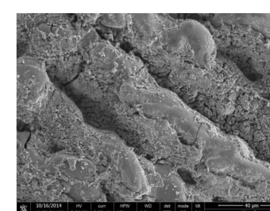
SEM of surface-modified LSM before (top) and after (bottom) isothermal aging, 700 °C/ 480 h
