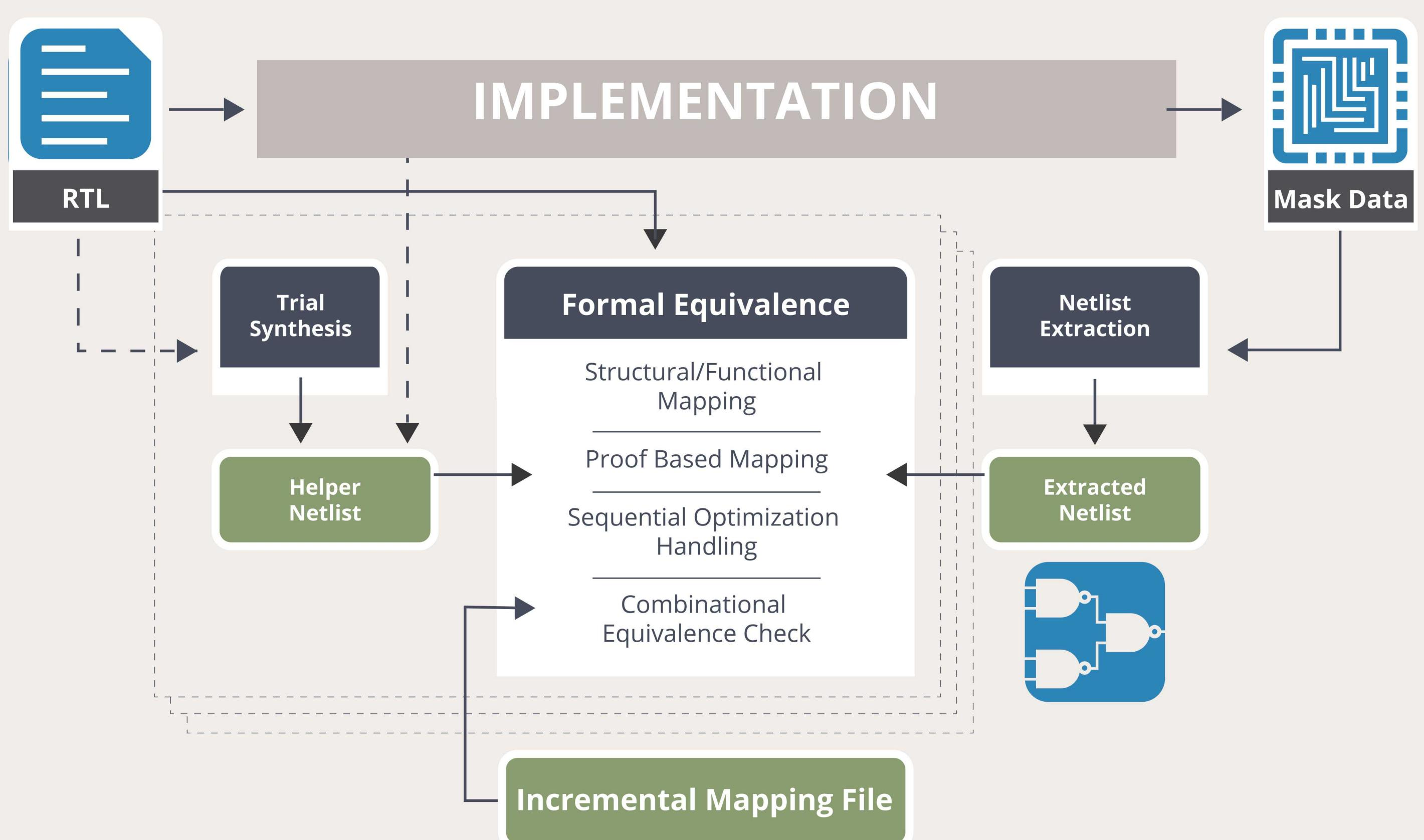
The black-box flow compares RTL directly to a netlist extracted from the mask data (GDS or MEBES).
