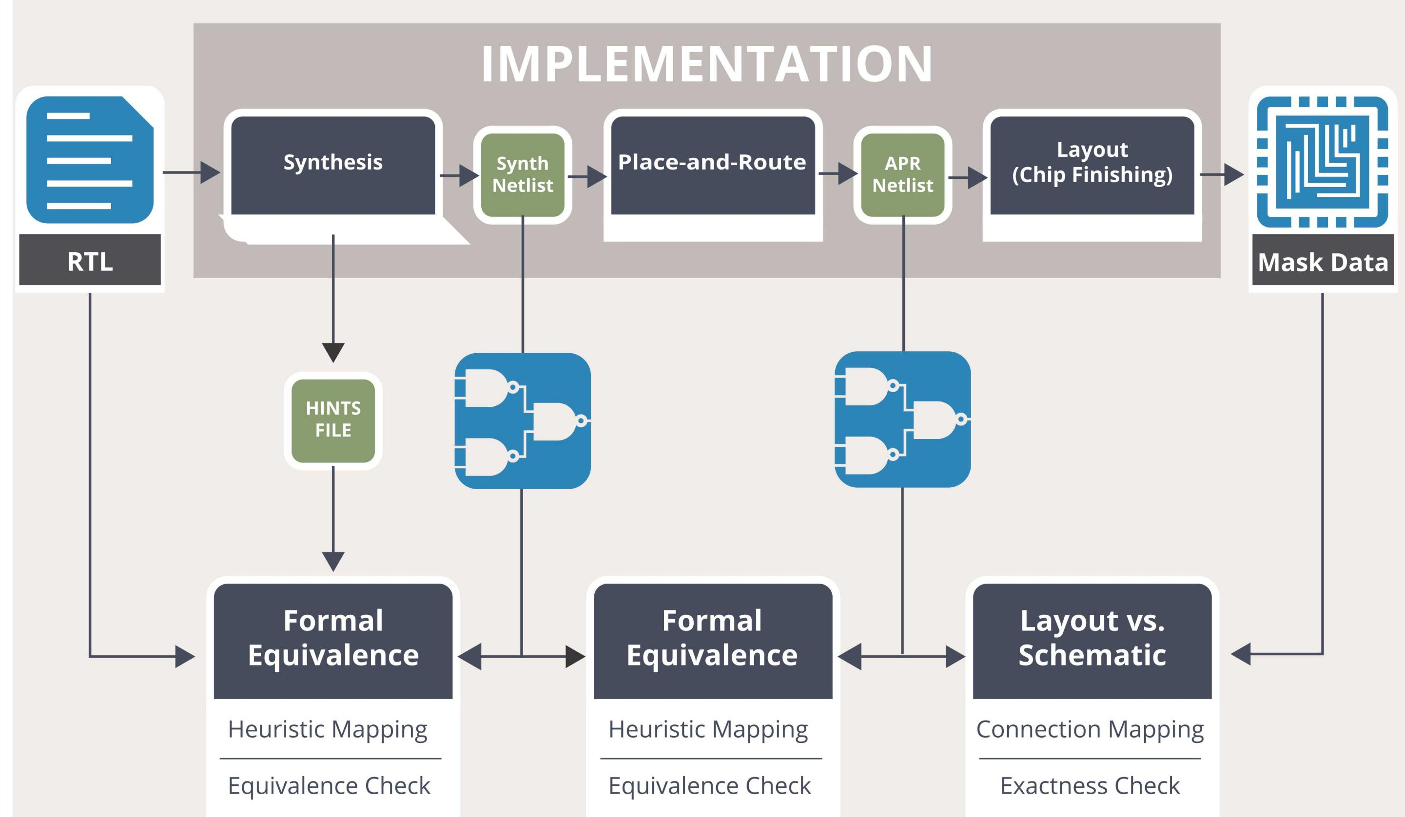
In the traditional equivalence flow, the implementation outputs are verified incrementally.
