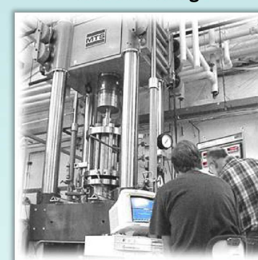
One million pound loading machine with triaxial pressure vessel.
