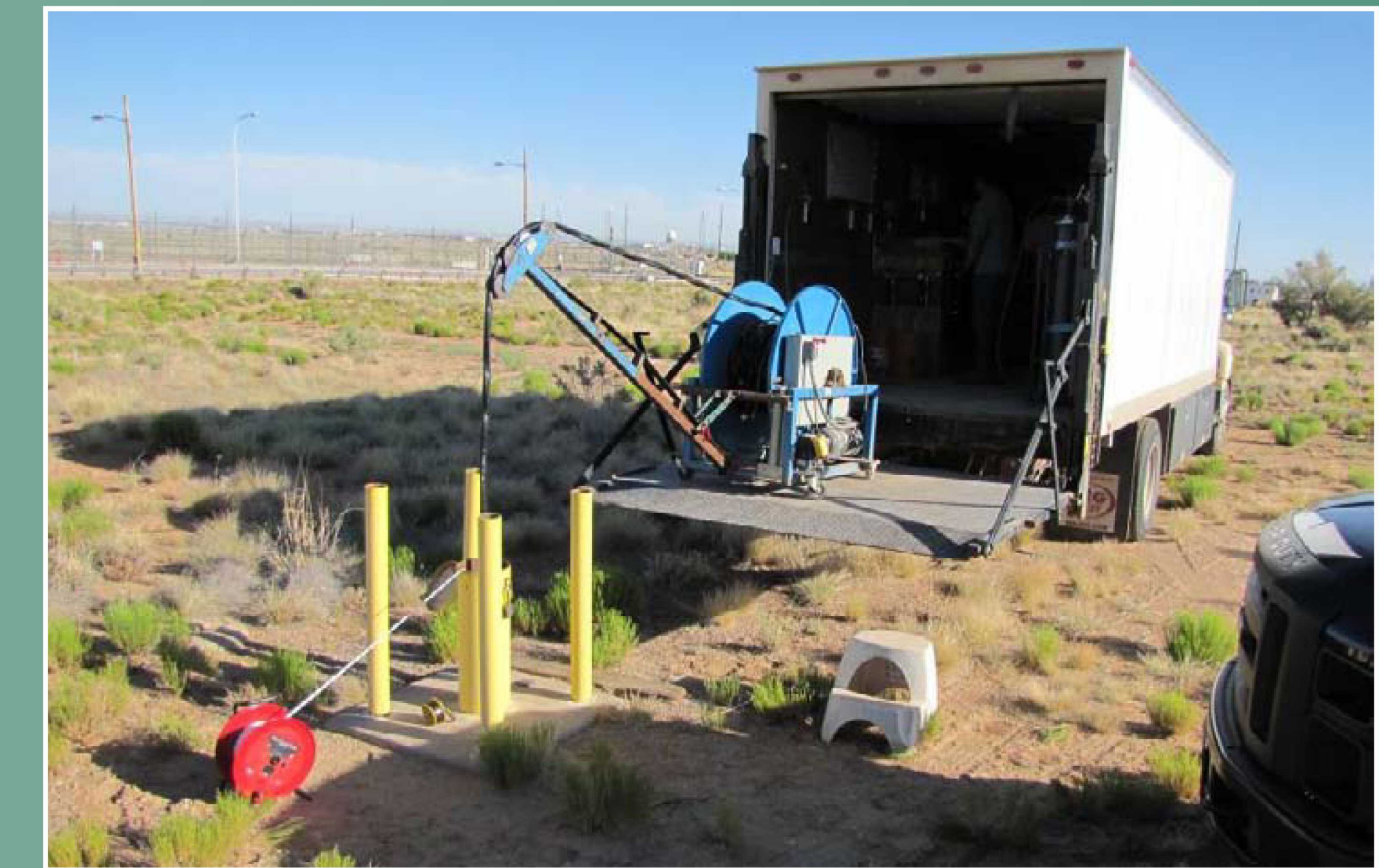
Groundwater monitoring truck with sampling pump and water level meter deployed in a monitoring well.
