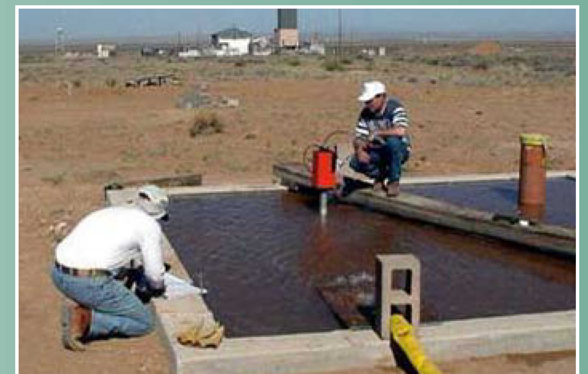
Field infiltration testing – results used for ET cover performance modeling presented in the CMI Plan.
