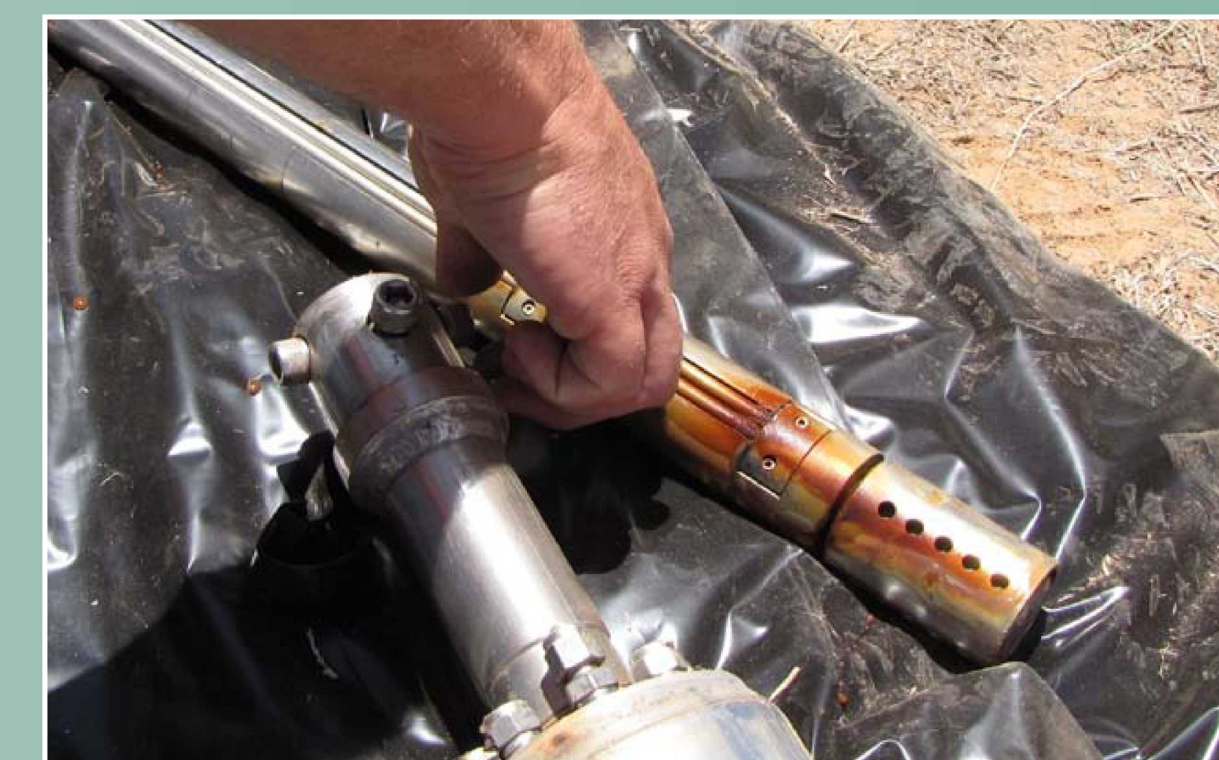
Visible corrosion of the MWL-MW4 dedicated stainless steel sampling pump when replaced in May 2009.
