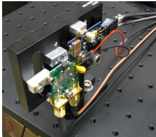
microfuzer with support electronics
