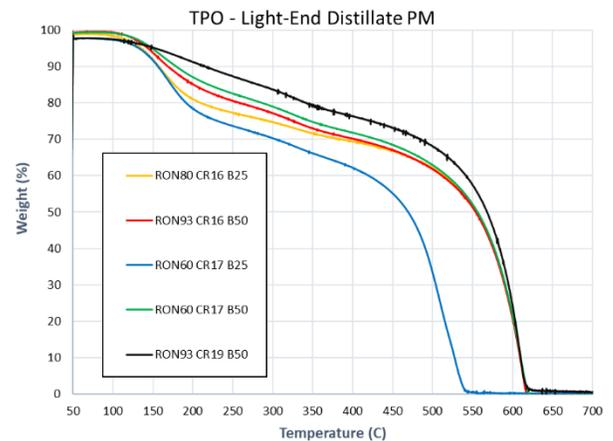
Figure 2. Normalized PM mass loss during TGA
