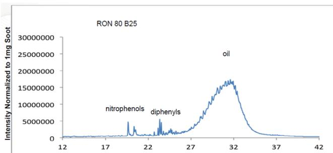
Figure 4. Non-polar HC species detected by TDU-GC-MS for ULSD and RON 80 PM samples
