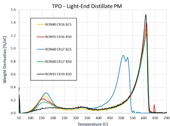
Figure 3. Derivative of the PM mass loss as a function of temperature
