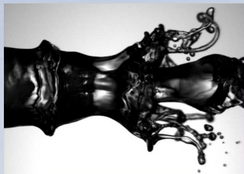
Liquid fuel spray break-up
