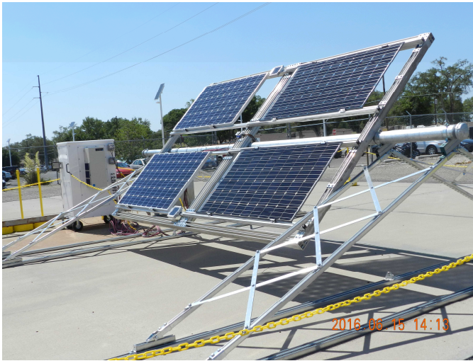
Fig 1. Sandia's adjustable, single modules IV curve rack in Albuquerque, NM. Two bifacial modules are on the right and two monofacial modules are on the left.
