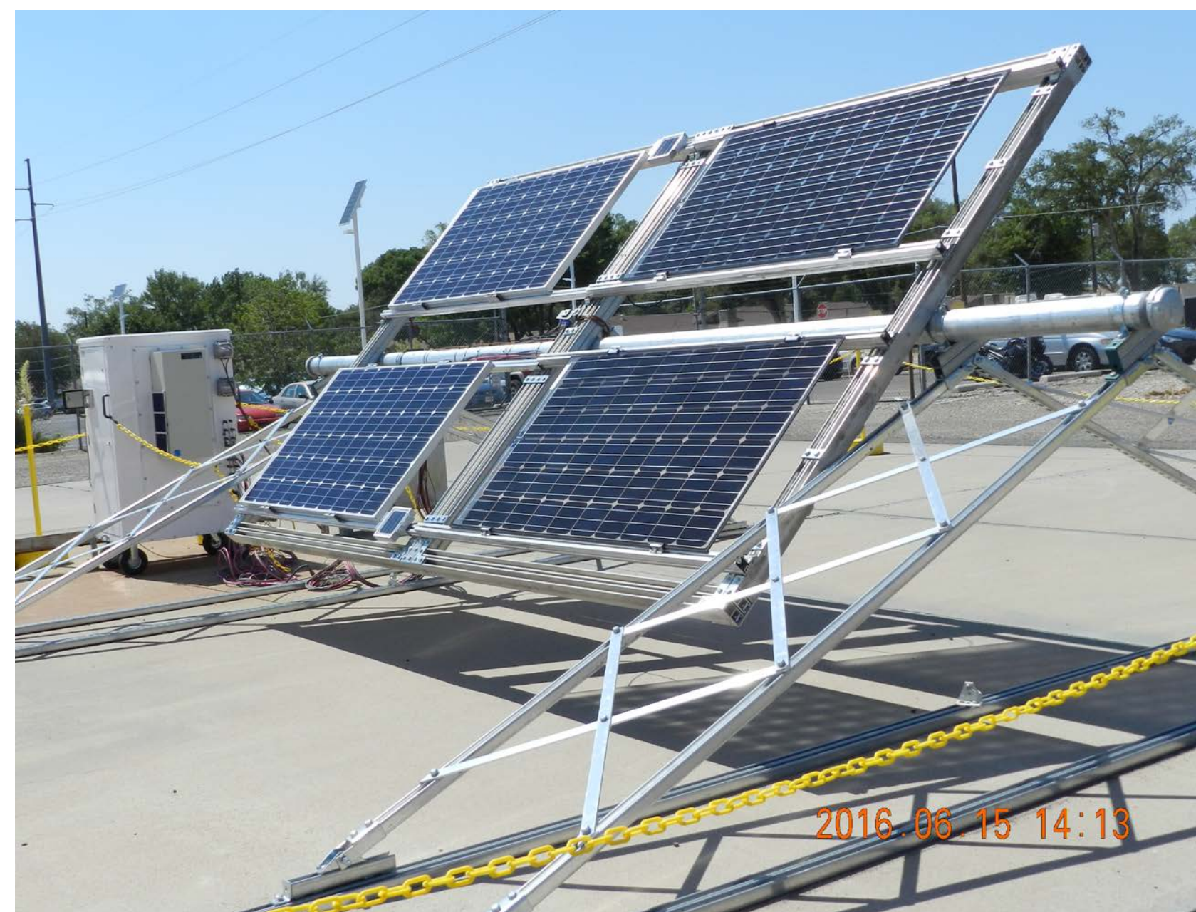
Single module IV tracing at different tilts and heights.
