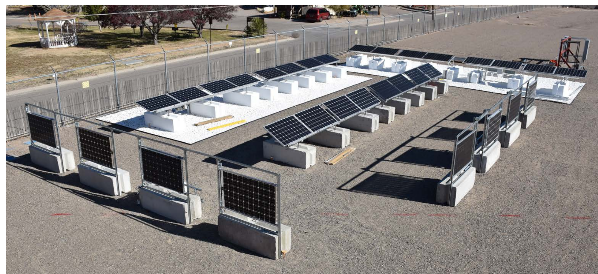
Single module monitoring on microinverters at five different orientations.
