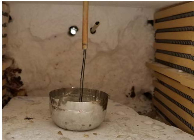
Figure 2.5. Furnace cool experiment with embedded thermocouple.
