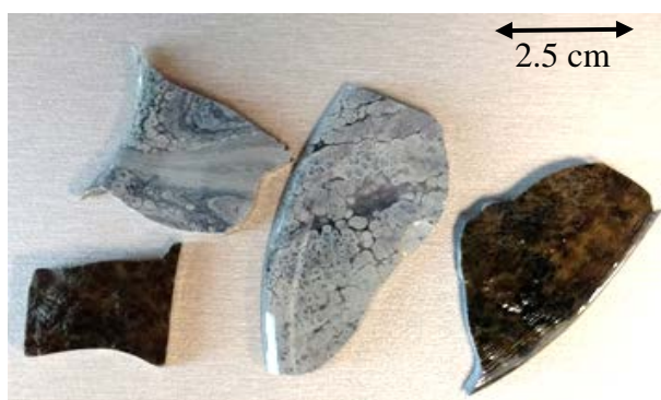
Figure 2.2. Optical image of the as-received glass. The darker side is the side of the melt that was in contact with the Inconel plate when the melt was quenched.
