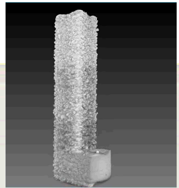
captured defect holes part CT image, Zeiss Xradia 520 Versa, voxel resolution ~ 2 \mu m, Harlan Brown-Shaklee
