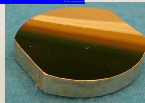
non-rotationally symmetric freeform mirror, Boye, Opt Eng , 2013
