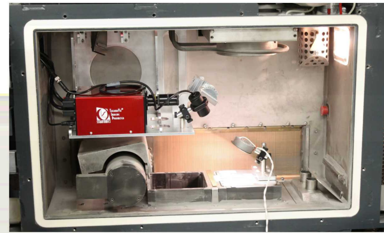
ThermaViz installed in the 3D Systems ProX 200
