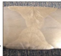
Weld zone, Ranor 304 SS plate
