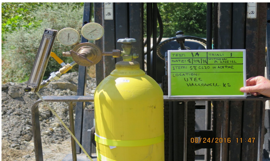
1(a) Air supply for bubbler (also used for the UN 2(a) tests).
