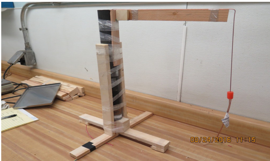
1(a) Setup showing no PMMA gap, detonation velocity probe, the bubbler tube is on the far side.
