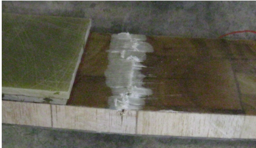
Figure 89: Beam 5 compressive face sheet failure.
