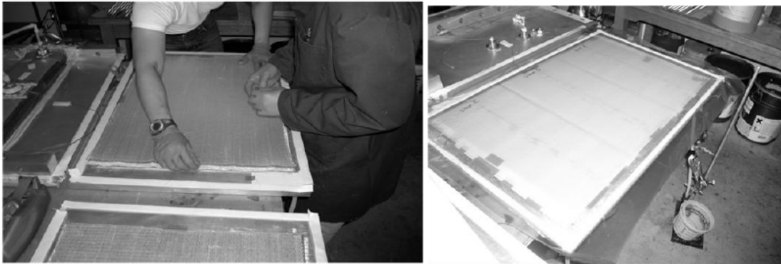
Figure 16: Preparing mold to inject resin to make laminate using vacuum resin infusion process. Laying materials on mold (left) and finished lay-up under vacuum (Nelson, 2013).
