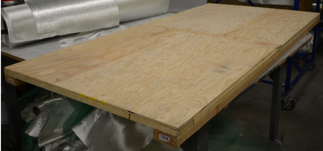
Figure 20: Table top with removable section for continuous fiber IP (CFIP) wave introduction.
