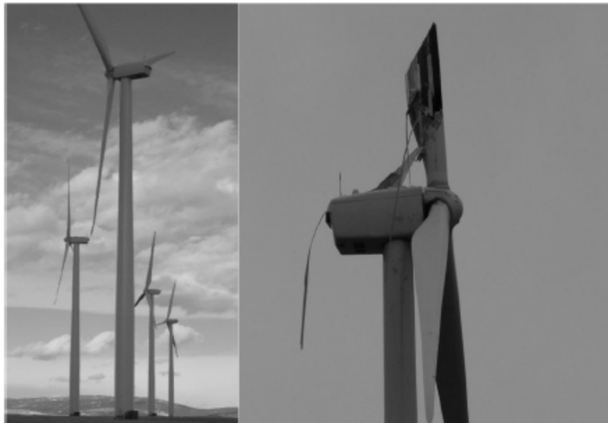
Figure 1: Typical wind turbine blades (left) and blade failure (right) (Nelson, 2013).
