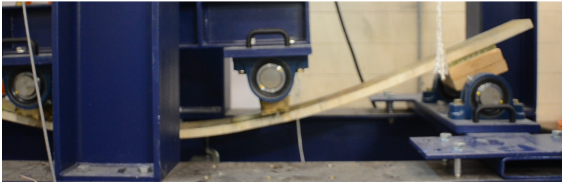
Figure 87: Beam 4 loaded and near maximum actuator travel reached by using wooden spacers shown.
