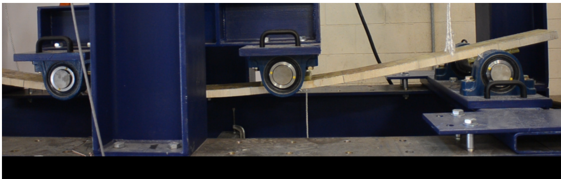
Figure 85: Beam 4 loaded and at maximum actuator displacement before adjusting to take advantage of full actuator travel.
