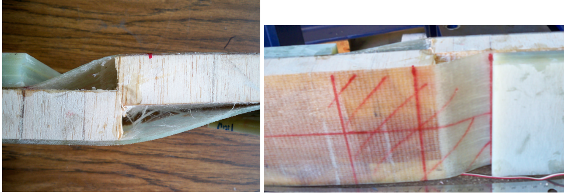
Figure 78: Beam 2 balsa shear failure and delamination.
