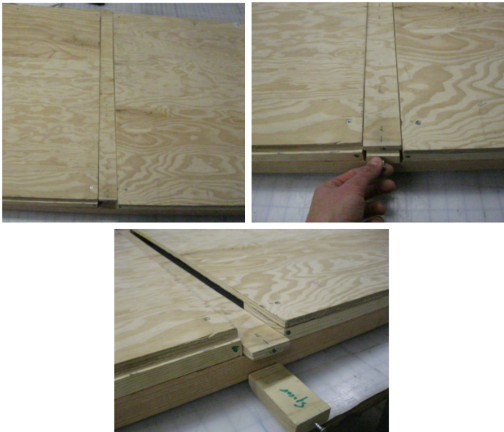
Figure 21: Table top middle strip. Removable middle strip (top left), spacer being removed (top right), middle strip dropped down after the spacers have been removed (bottom).
