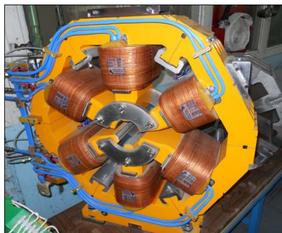
Figure 2. Typical segmented-pole design of a sextupole magnet.
