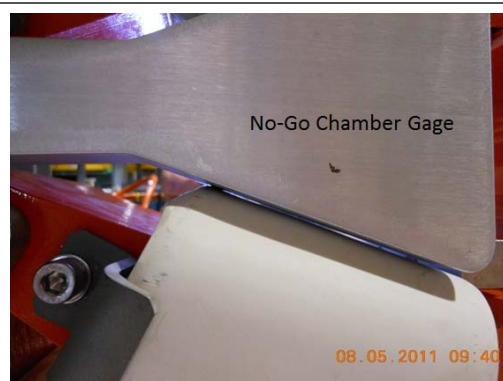
Figure 11: Coil to chamber interference check with a no-go gage block.
