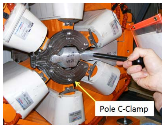
Figure 12: An assembled pole c-clamp for a sextupole magnet.
