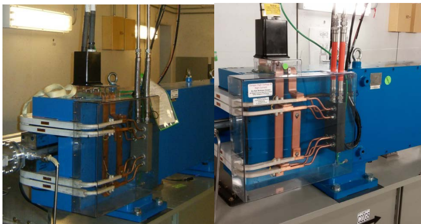
Dipole magnet with stainless steel braided hose connection(left) and radiation resistant rubber hose connection (right)
