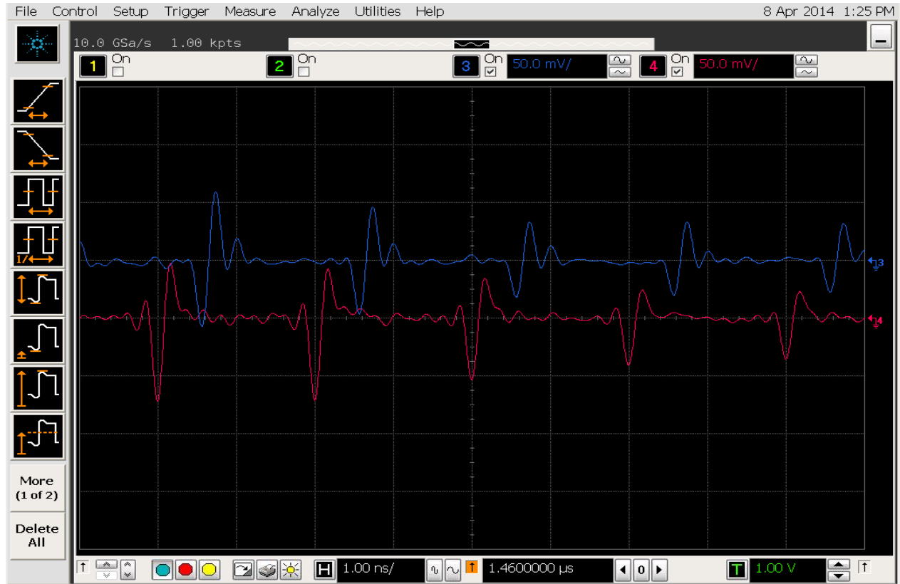
Figure 2, raw button signals for TMS, notice the pulses are not arriving at the same time due to cable length difference.
