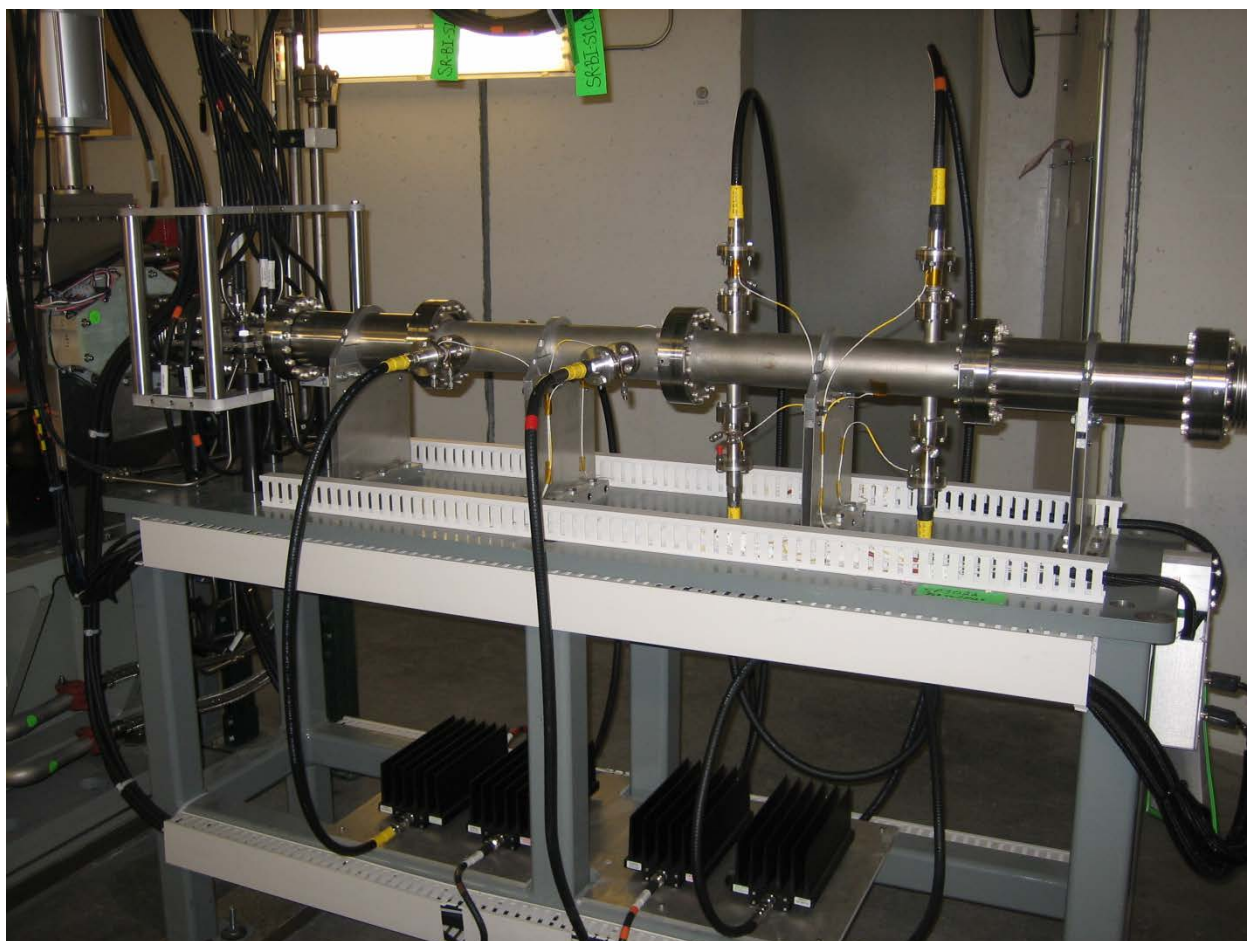
Figure 5-2, Stripline kickers in the storage ring tunnel.
