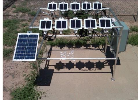
*Electrical Performance Sampling Station. Set-up used to determine performance loss due to natural soiling processes*
