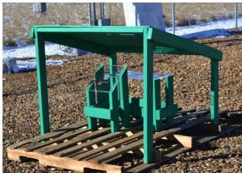
*Atmospheric Particulate Sampling Station. Set-up used for the collection of airborne particulates that settle naturally.*
