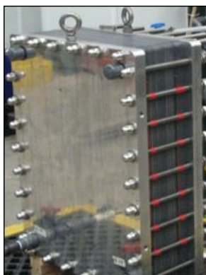
Figure 18: Ashlawn Energy vanadium redox flow battery 10 kW Stack [14].
