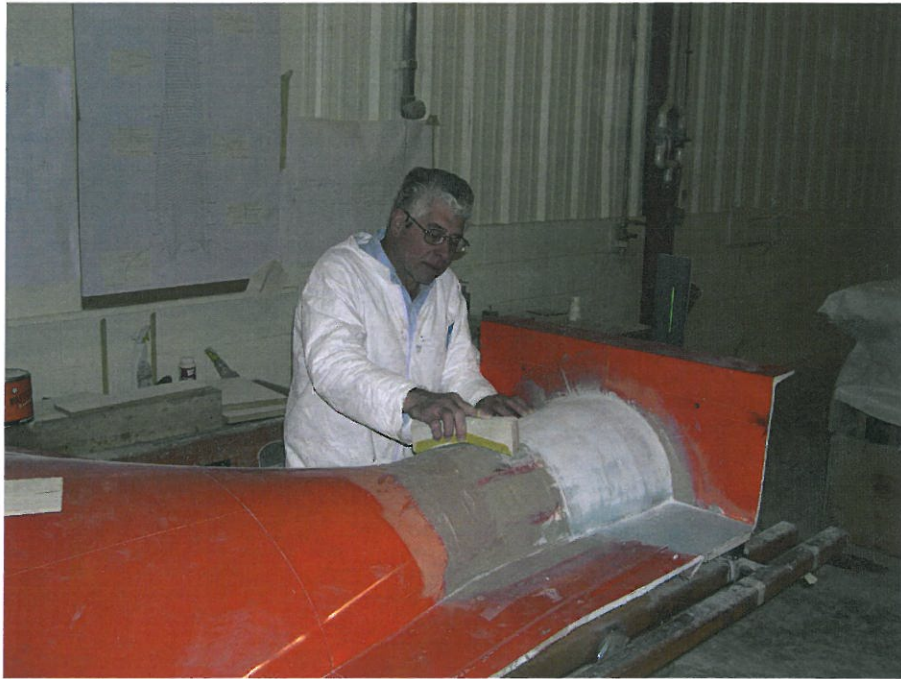
Figure 21 CX-100 Root Sanding
