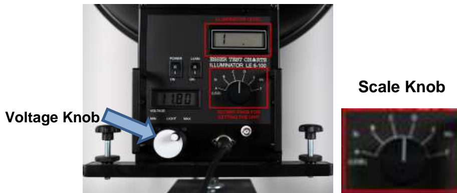
Figure 36. Test Chart Illuminator Showing Scale Knob Position and Lux Meter
