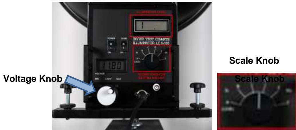
Figure 56. Test Chart Illuminator and Close-up of Scale Knob
