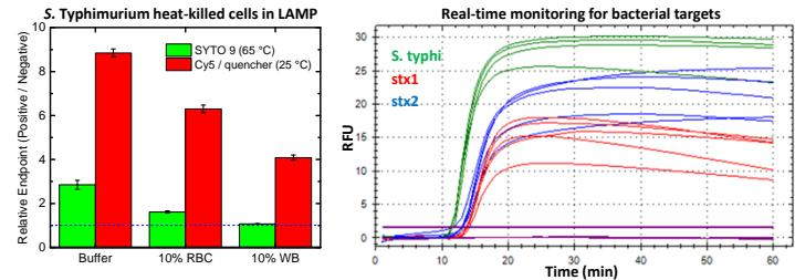
**LAMP in a microfluidic sample analysis platform:** The combination of sensitive, specific detection, extraction-free sample prep, tolerance to crude samples, and low operating cost makes LAMP ideal for implementation in low-resource settings. Our novel single-step closed-tube detection technique extends this capability by providing easy discrimination between positive and negative endpoints and multiplexing capability.
