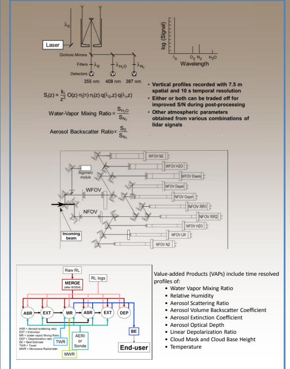
SGP Raman Lidar
