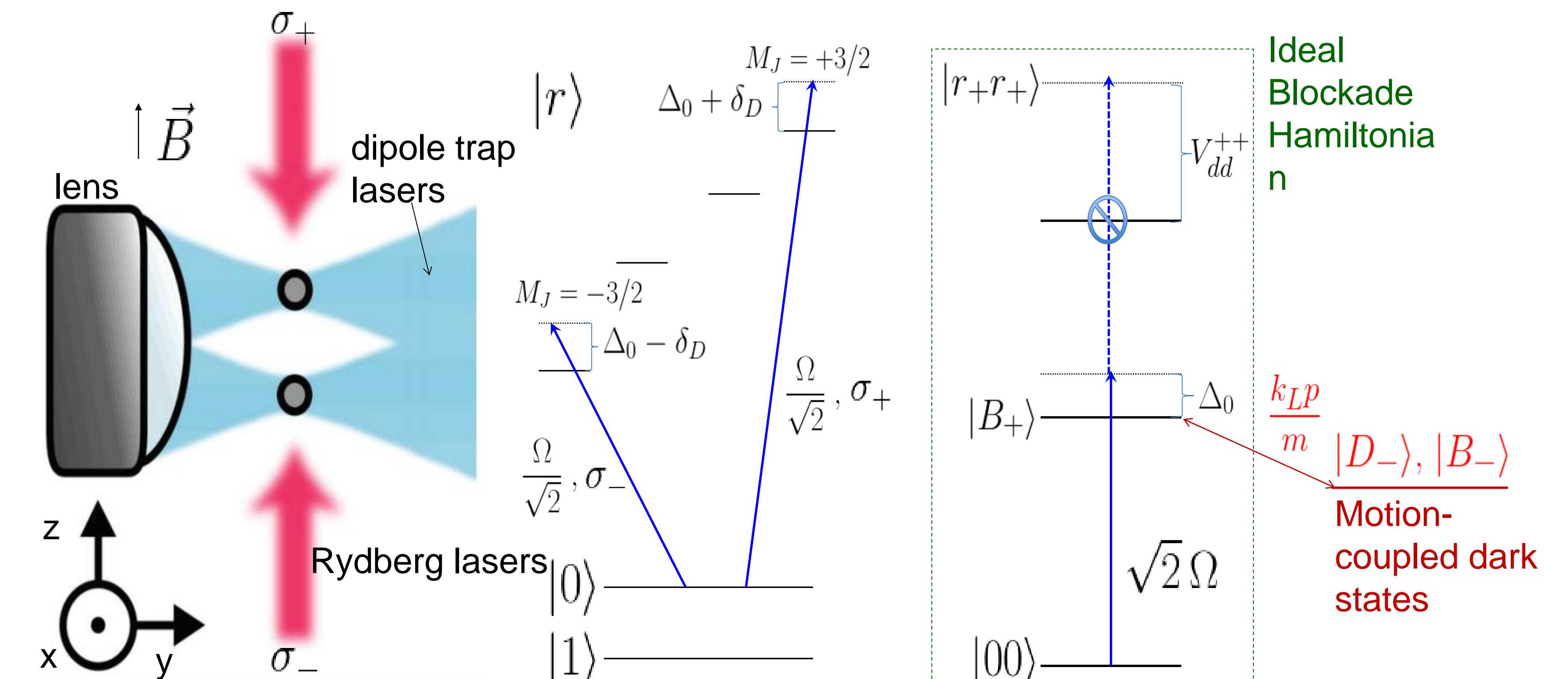
The trapped atoms are illuminated by two counter-propagating lasers, with equal frequencies but opposite base detunings but opposite Doppler shifts.
