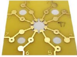
(Left) Photo of individual lens showing eight electrodes forming a central confinement region. (Right) Photo of the assembled device integrated with an electro spray ion source.
