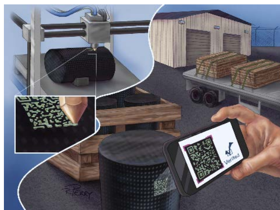
Using a QR code printed onto a part to validate its authenticity.
