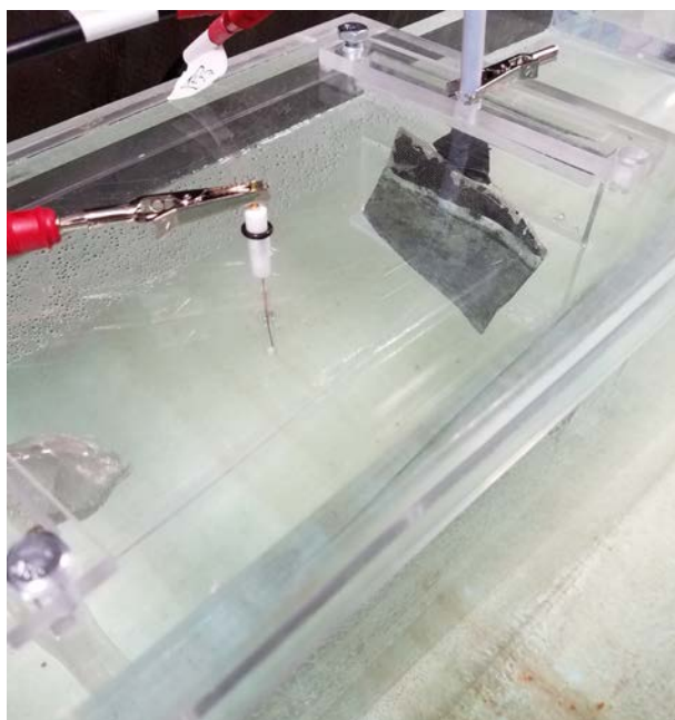
The electrochemical system used for testing in the raw seawater flume at MSL.
