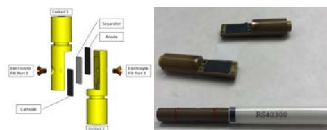
In situ MAS-NMR rotor cell design (left) and an actual cell photo (right).
