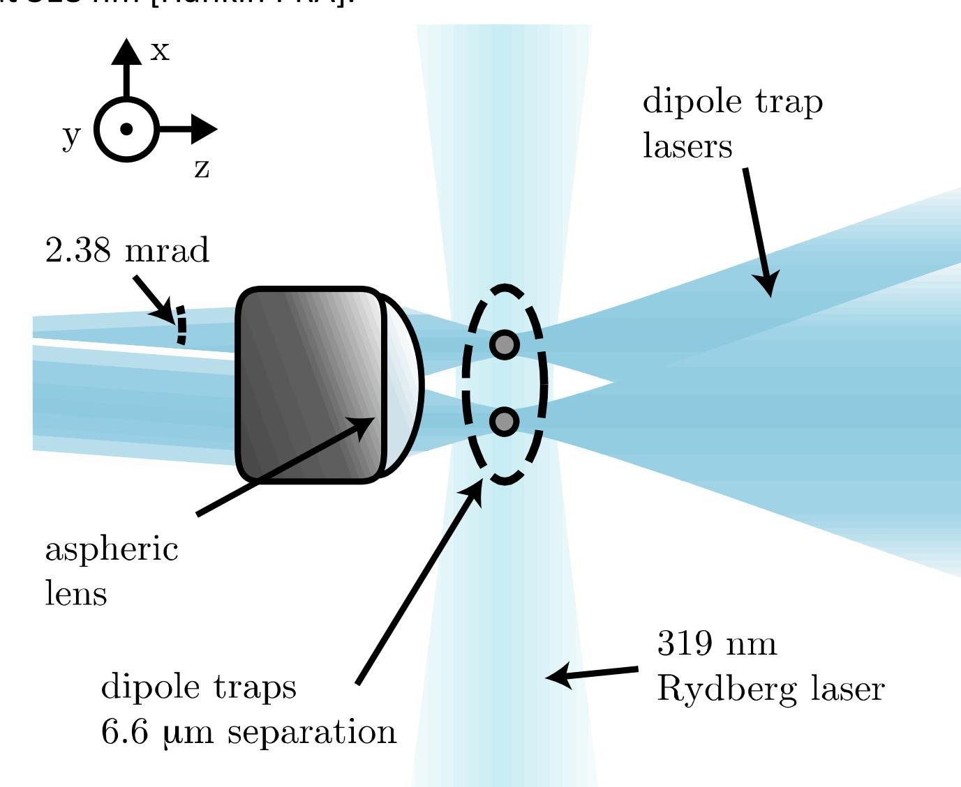
We trap single cesium atoms in optical dipole traps formed by focusing two 938 nm laser beams through a high NA aspheric lens. The relative angle between the two beams is chosen such that the two traps are separated by 6.6 mm during atom loading. We dynamically tune this parameter in our experiment to tune the interaction.
