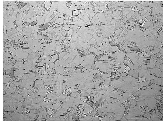
(b) 304 SS Un-Shocked Sample (100X)
