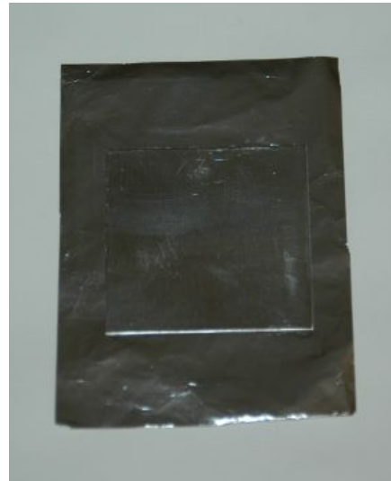
(a) 0.030 cm (0.012") Flyer Layer (b) 0.033 cm (0.013") Composite Flyer Assembly
