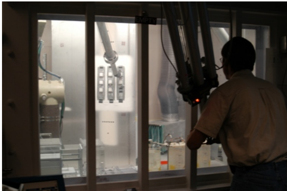
Figure 3.3: Remote Handling Operations Using Master/Slave Manipulators
