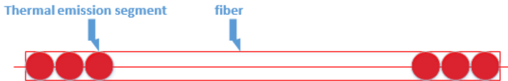
Figure 67. Thermal emission in sapphire fiber.
