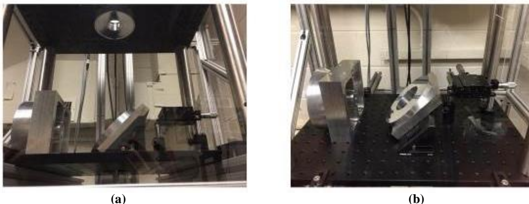
Figure 8. The layout of the growth chamber accommodates the presence and movement of the feedstock and fabricated sapphire fiber while focusing the laser light into a central hot zone.
