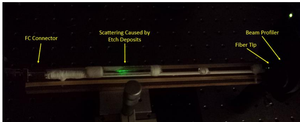
Figure 33. Aluminum sulfate/phosphate deposited on fiber surface at a concentrated location during etching causes significant scattering loss, visible using a 532nm green laser.
