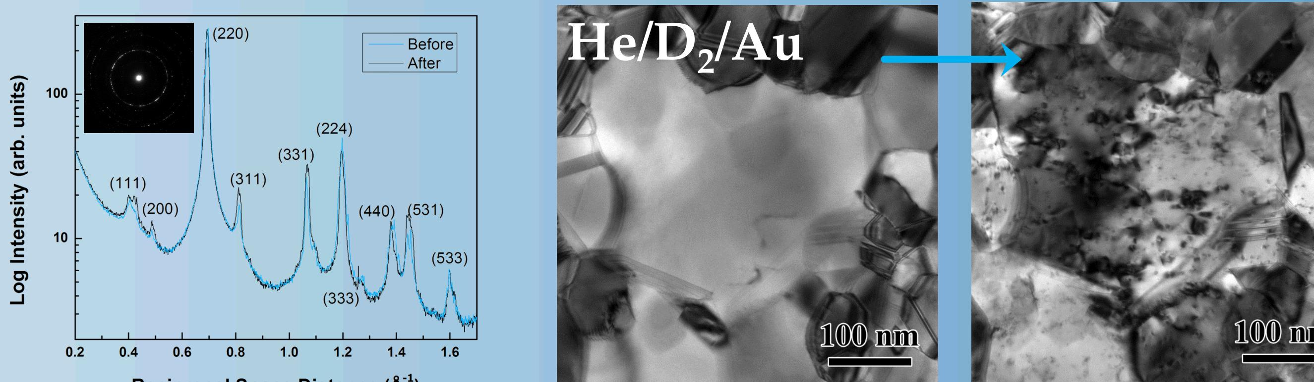
(left) Peak intensity changes in averaged selected area electron diffraction patterns, (right) accumulated damage as a result of the implanted components
