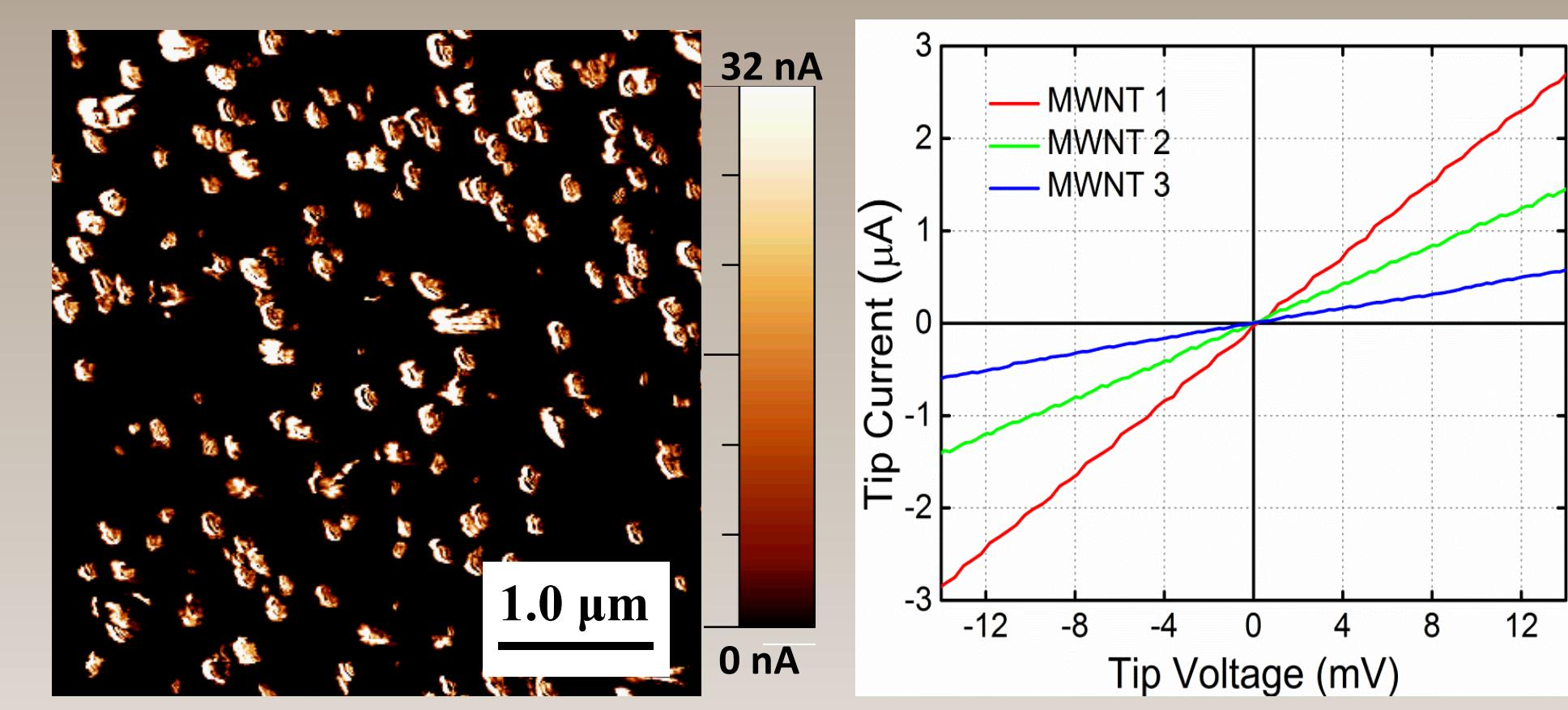
Conductive AFM confirms electrical (and therefore thermal) contact to the substrate is preserved.
