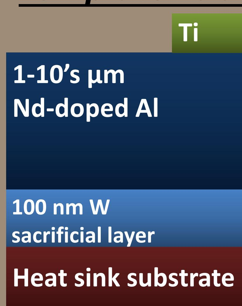
Anodize exposed Nd-doped Al to form pores.
