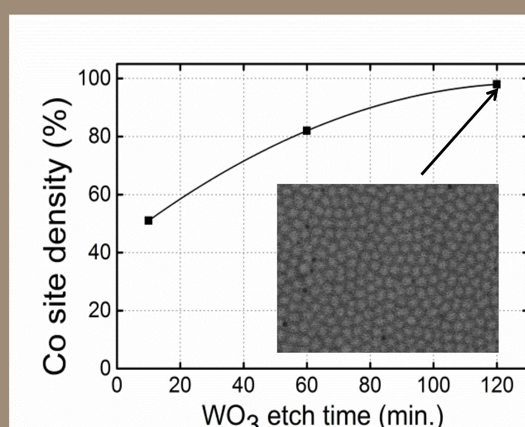
Inset: top view of filled pores flush with template surface
