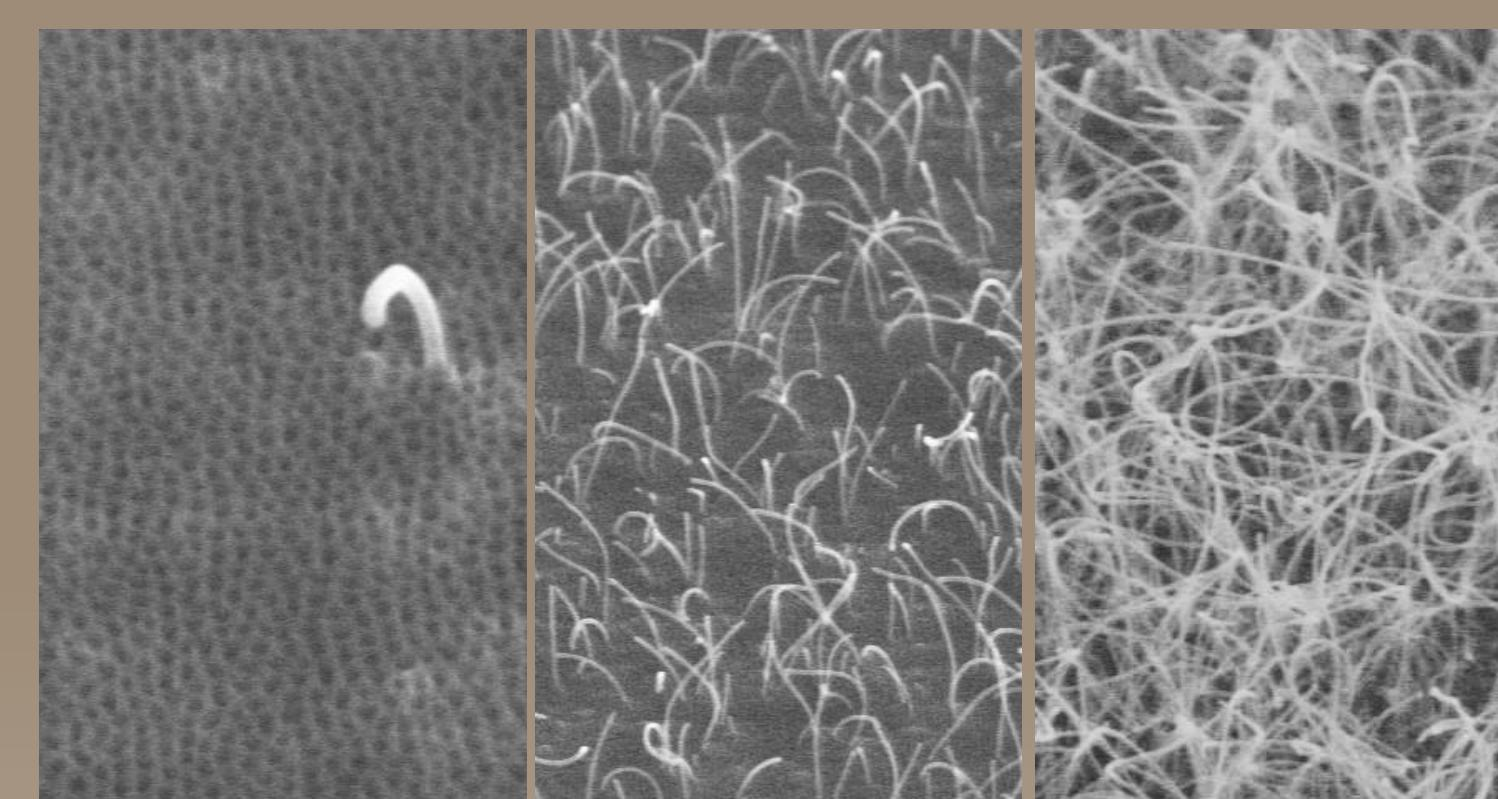
Nanotube density varies with the aspect ratio of the open pore above the Co
