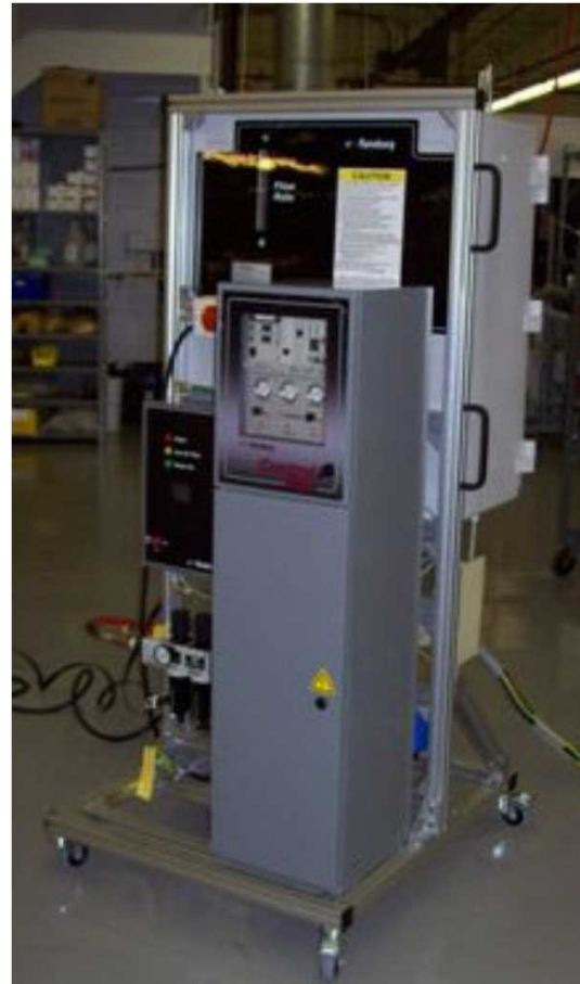
Rotary atomizer for aerosol delivery of decontaminants
