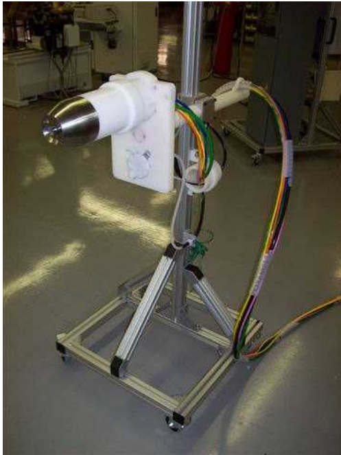
Rotary atomizer for aerosol delivery of decontaminants
